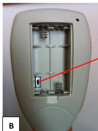
**Figure 2 A:** Display of the Jamar dynamometer. **B:** selector switch.
